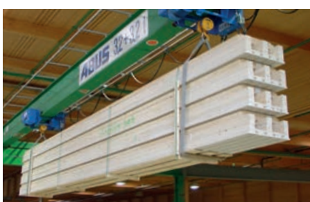
Finished joined BV box elements
