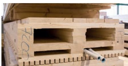
Ex works installation of conduits at the level of an additional layer \_p26
